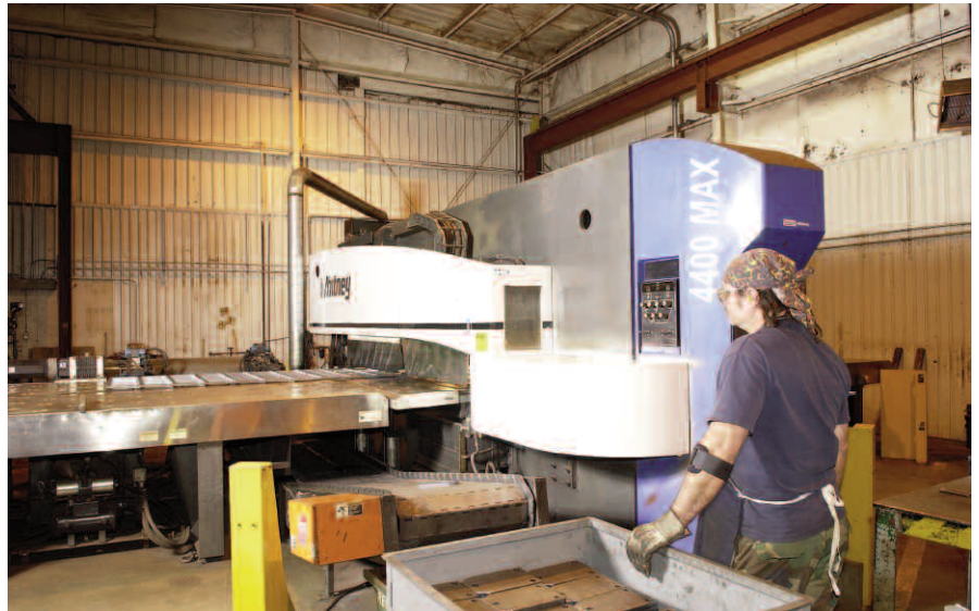
The majority of metal components over 1/2" thick that go into a Great Plains agricultural implement begin their fabrication process on the Whitney 4400 MAX. Operator Larry Shepherd monitors production.
