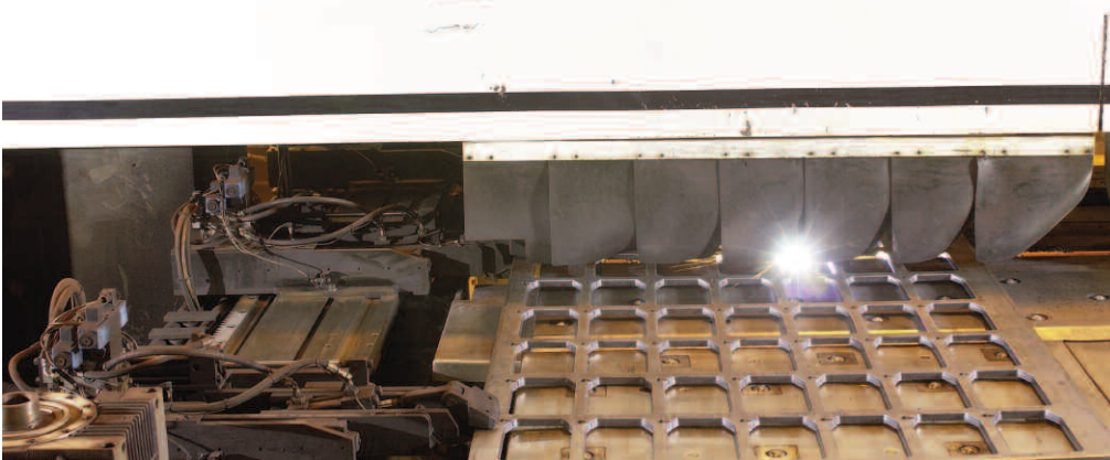
Three retractable, independently controlled workclamps, optional for the 4400 MAX, allow use of the entire plate.
