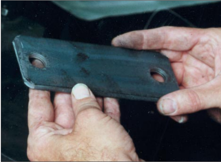
The 1524 CNC adds corner radiuses to 75 percent of the parts run on the machine. A standard tool from W.A. Whitney is used to produce the corners.
