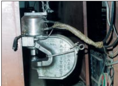
Marshall Erdman & Associates punches wide flange beams and other structural components with a pair of W.A. Whitney 100 ton capacity flange and web presses.
