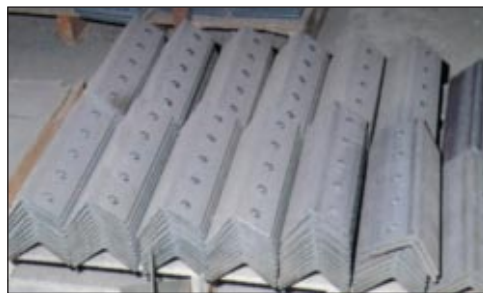
Base plates and clip angles punched for welding and assembly into structural components
