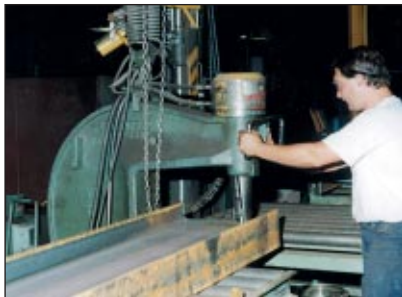
Interior and exterior wall sections being fabricated on a special line.
