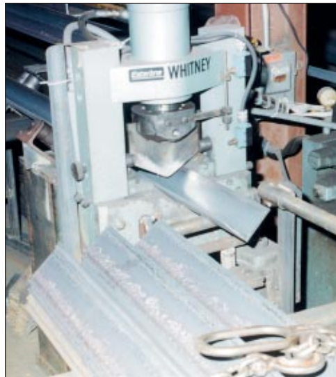
A Model 7609 W.A. Whitney 59 ton hydraulic angle shear is used for shearing bracing angles, clip angles, truss components, and other miscellaneous parts used in Erdman building fabrication. The shear is equipped with infeed/outfeed material handling and part length gaging.
