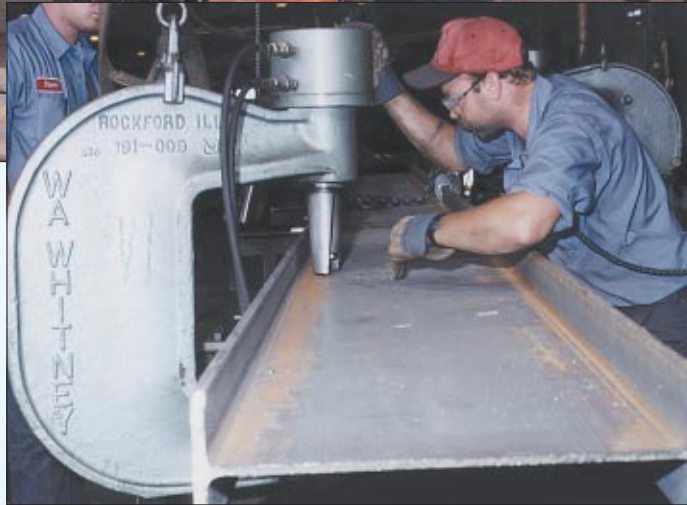
McFarlane's operator punches holes in wide flange beam with a Model 761, 90 ton capacity W.A. Whitney web style press.
