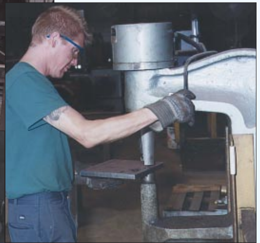
Operator at McFarlane Mfg. punches base plates utilizing a Model 791 Whitney press as a stationary punching press.
