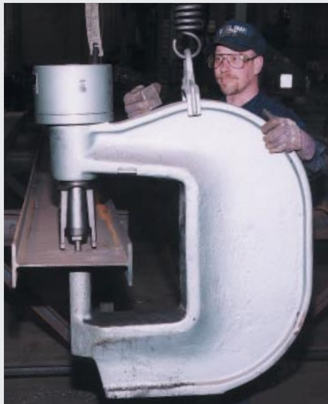
A jib crane and spring are used to bring the Model 791 Web Press to the beam for efficient punching.
