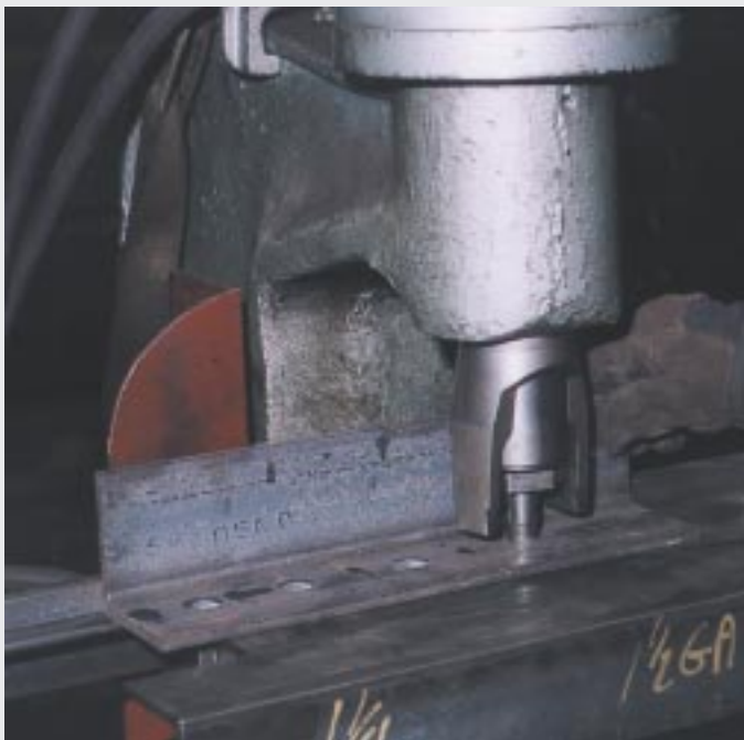
A Model 771 Web Press is held in a table fixture for punching clip angles. The press can be easily removed for use as a portable.
