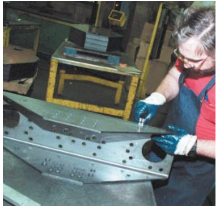
Nesting software compatible with the Whitney and the lasers helps operator Spencer Scott maximize material usage (left). Kenney Stephens, press brake operator, checks tolerances after a part from the Whitney is folded.
