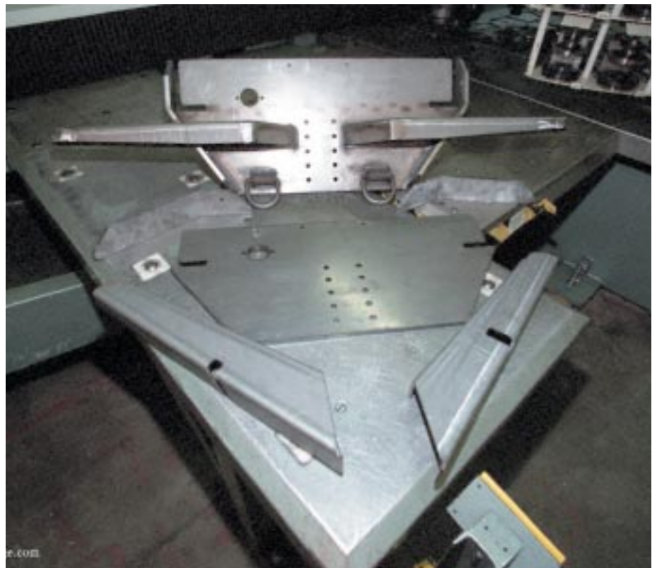
A kit of parts and its assembly. Final product is a hitch plate for a one ton truck for one of Voisard's many municipal customers.
