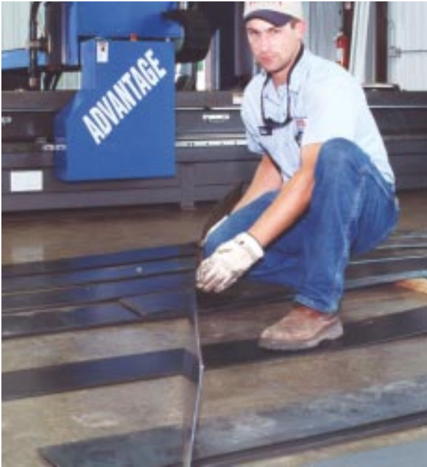
ADVANTAGE Operator Chris Fontenot shows edge quality. The clean edges allow parts to go directly to welders like Kerry Steyer without an additional clean-up operation.
