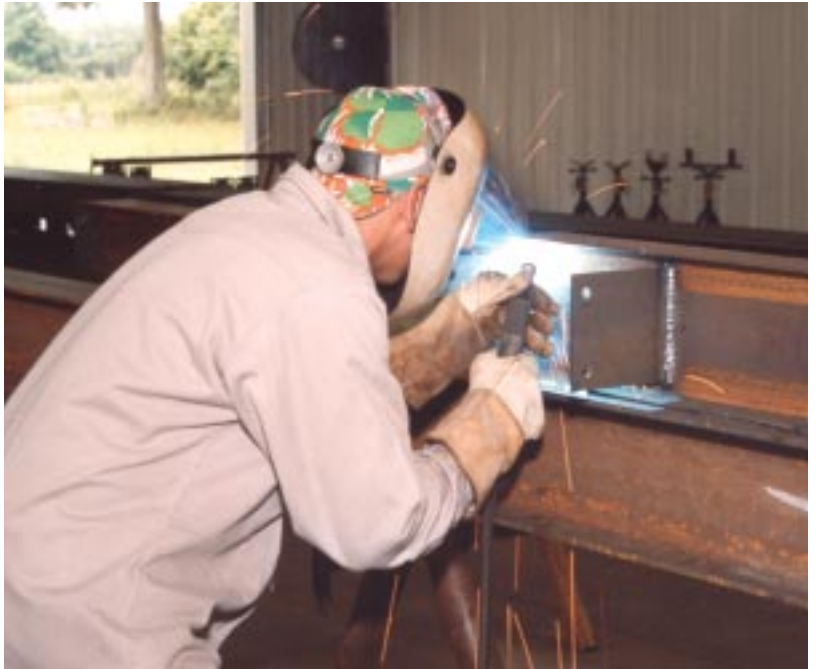
ADVANTAGE Operator Chris Fontenot shows edge quality. The clean edges allow parts to go directly to welders like Kerry Steyer without an additional clean-up operation.
