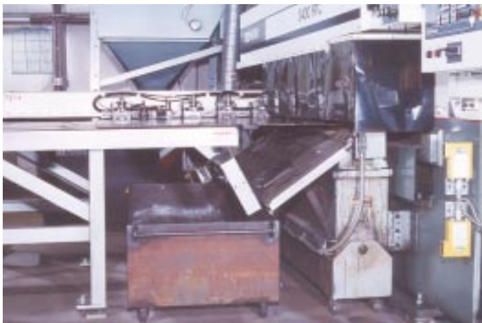
A Drop Door Retrofit package, added in Spring of 2002, increased production by 25 to 30 percent.
