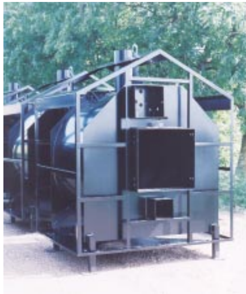
Critical tolerances are required for internal and external stove parts. The robotically welded tanks hold up to 180 gallons of water. Parts from material from 1/4" to 3/8" —including the identifying "JOHNSON" for the doors—are produced on the 3400 RTC.
