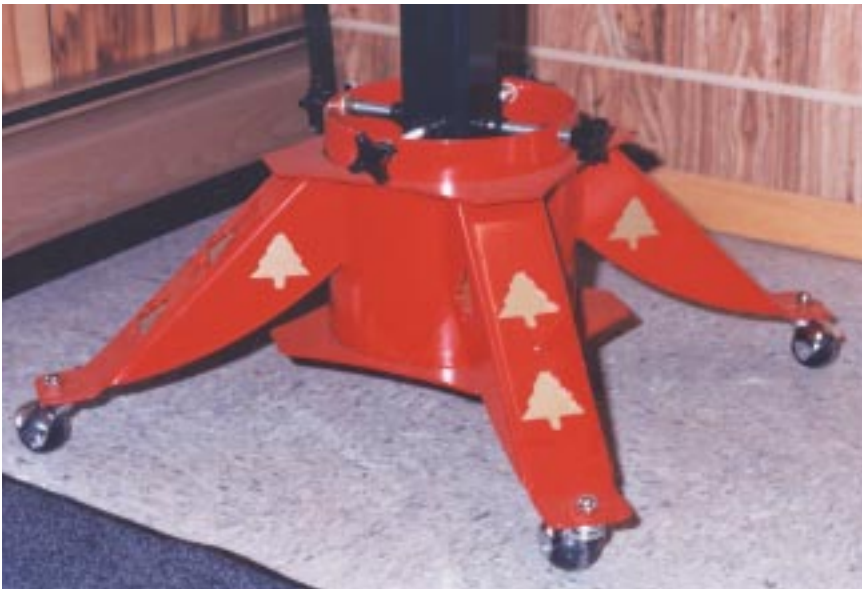
Goerke and Kris Puffer, his daughter, show the heavy-duty construction of the Lifetime tree stands. All parts except the 3/16" tubes are cut on the Whitney.
