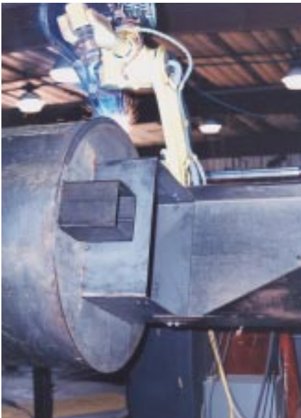
Critical tolerances are required for internal and external stove parts. The robotically welded tanks hold up to 180 gallons of water. Parts from material from 1/4" to 3/8" —including the identifying "JOHNSON" for the doors—are produced on the 3400 RTC.
