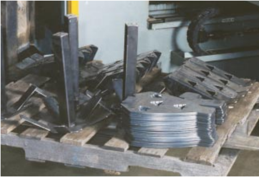
Production parts for Pro-Weld's proprietary line of Lifetime tree stands go directly from the 3400 RTC to a press brake or weld station.
