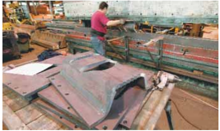
Bucket parts are first cut on the PlateLASER-II. Holes are reamed for size and surface finish. After forming, parts are trimmed using layout lines previously engraved with the PlateLASER-II.
