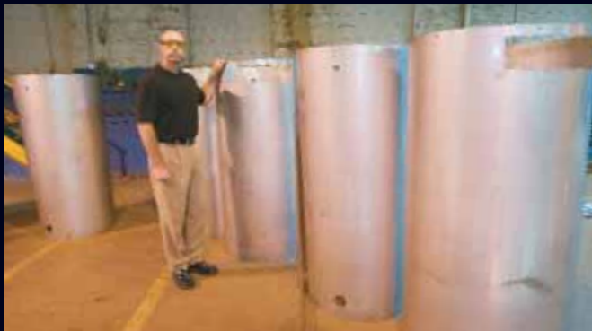
16 gauge stainless steel shells for heat exchangers.
