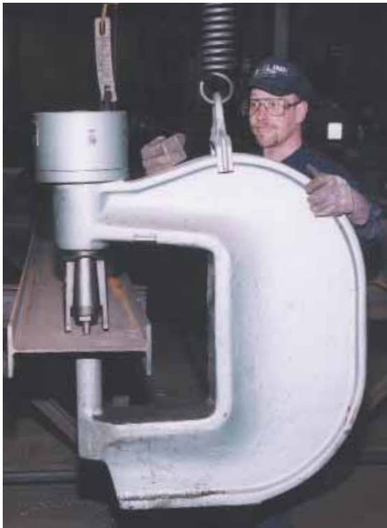
A jib crane and suspension spring position the 90-ton Model 791 Web Style Press to layout points on a wide flange beam.
