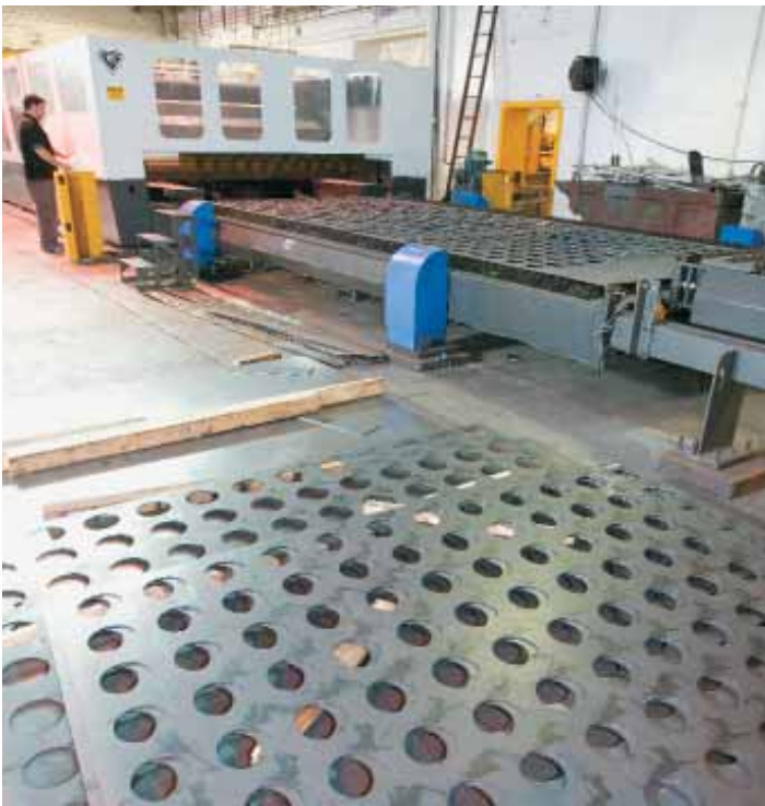
Tube sheets, 92" wide. Three parts made from one sheet 240" long with 336 5" diameter holes.
