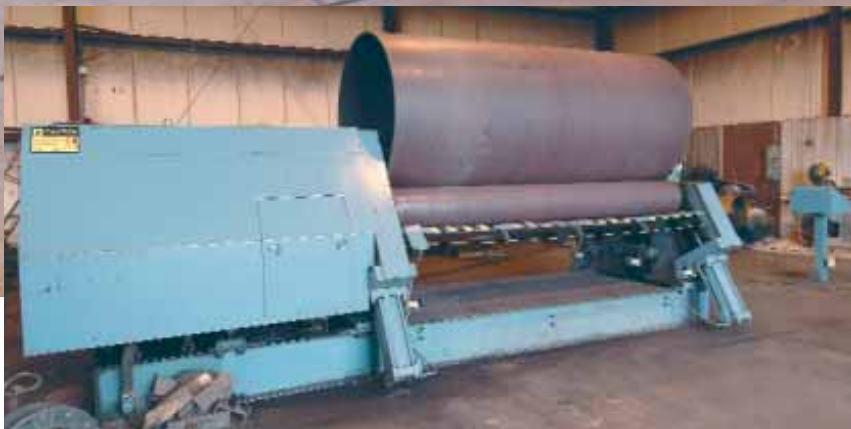
Bertsch roll forms pre-bend up to their full capacity. Here, operator Steve Kincaid rolls 10' wide 1/2" A36.
