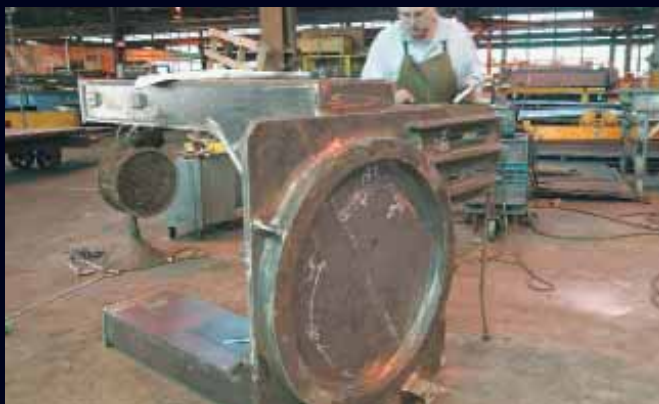
Steering yoke weldment. Welds are critical and require ultrasonic and magnetic particle testing.
