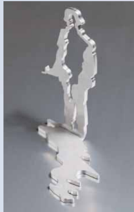
Statuette from dinner sponsored by National Vietnam Veteran’s Art Museum honoring inaugural “Above And Beyond Award” recipient Gary Sinise. Figures were cut from 1/4" stainless steel on PlateLASER-II.
