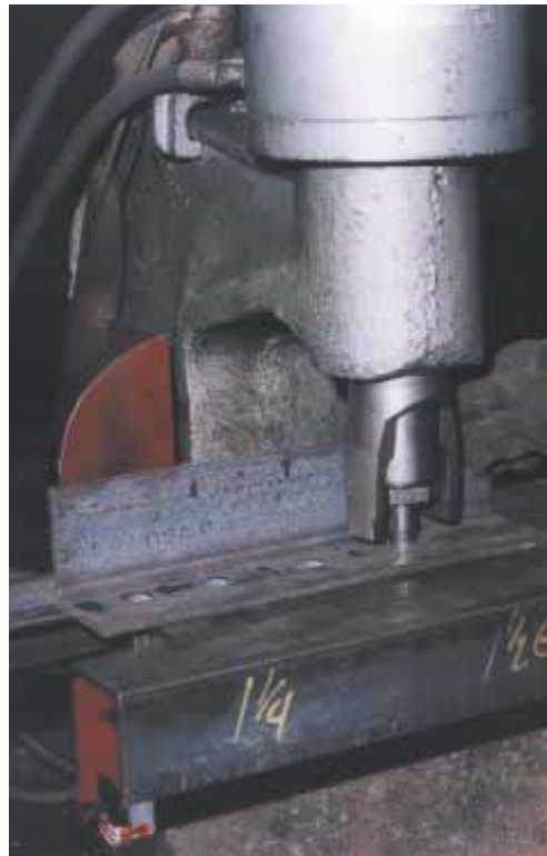
A Model 771 Web Press is held in a table fixture for punching clip angles. The press is easily removed for use as a portable.
