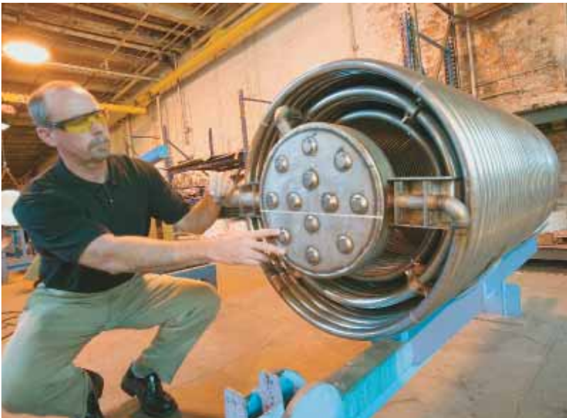
Heating coil for de-icing units. Stainless steel tubing must be rolled to exact tolerances. Randy Hauser points out the bulkhead cut from 1/2" stainless on the PlateLASER-II. Machining operations were eliminated on this part with the PlateLASER-II.
