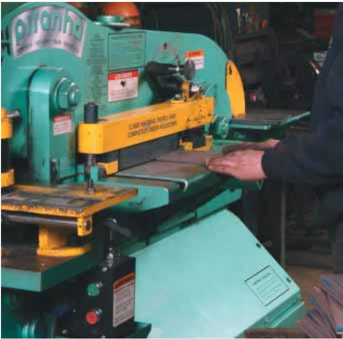
The coper-notcher capability on the P-50 is used virtually everyday—faster and more accurate than any previous process.
