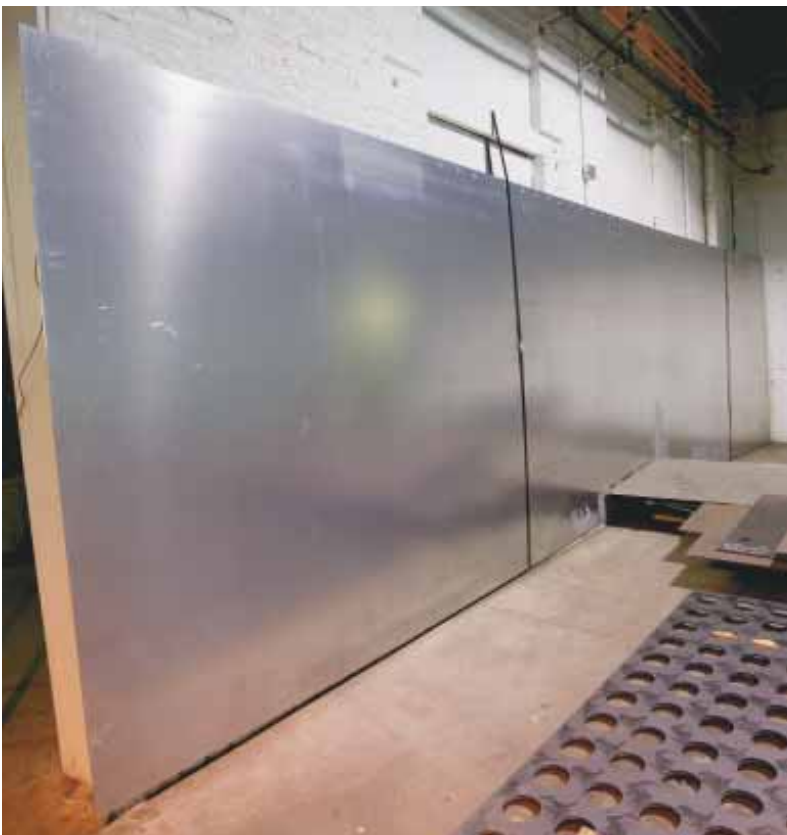
Rail car side — 95" x 35' with 1100 holes in 3/8" aluminum.
