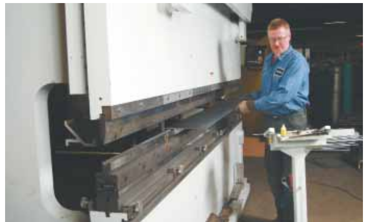
The automated backgauging system eliminated double handling of parts. For some jobs, production time is now a third of what it used to be.
