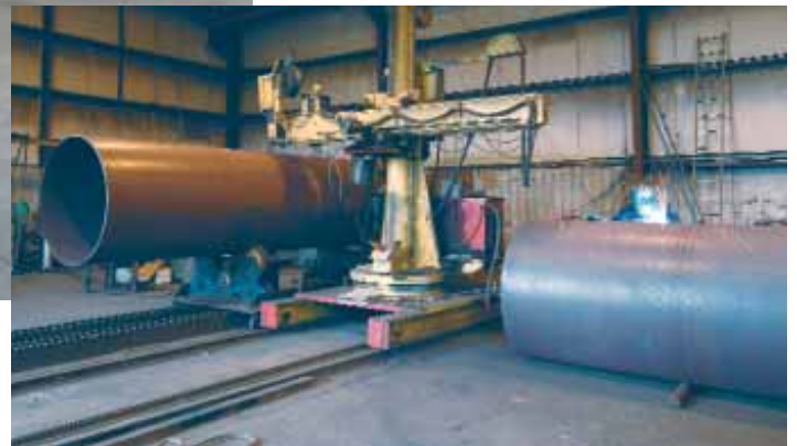
The speed of the four roll Model 87-10 impressed Anthony Jurkas, owner of Universal Pipe & Supply in Joliet, IL. Pipes from this job are joined by welder Rodolfo Diaz into 20' sections for the road boring industry.
