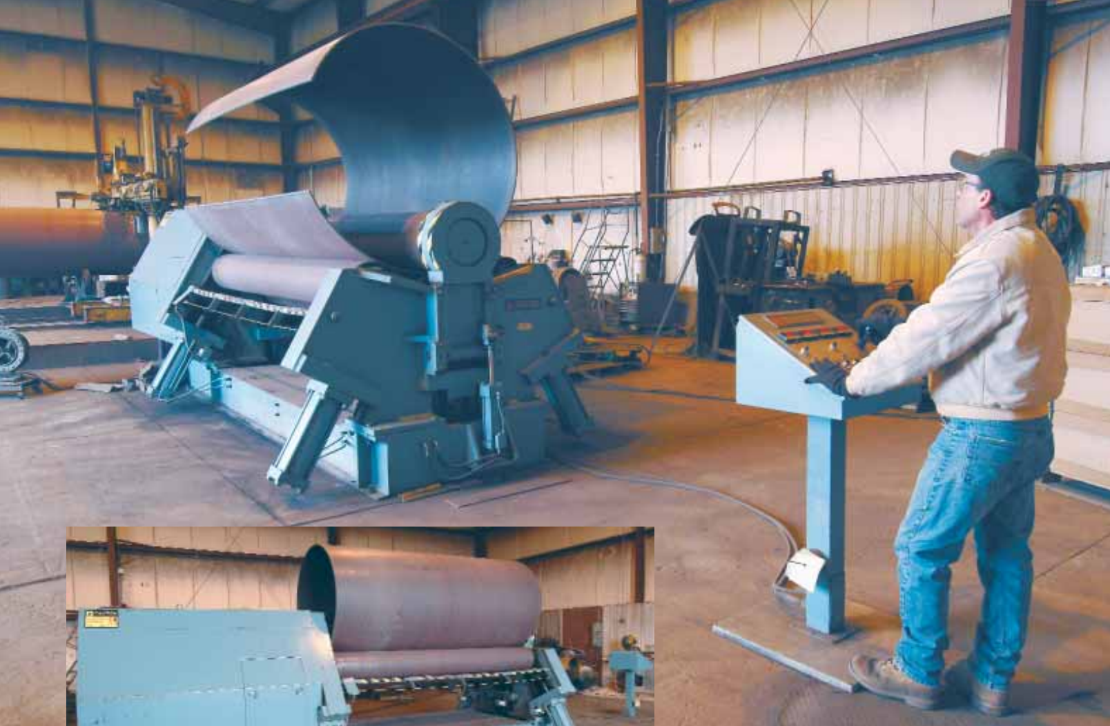
Bertsch roll forms pre-bend up to their full capacity. Here, operator Steve Kincaid rolls 10' wide 1/2" A36.
