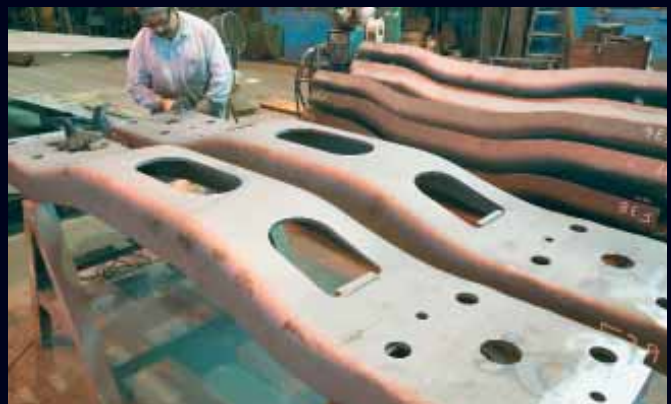
High speed rail car parts. All welds require X-ray inspection.
