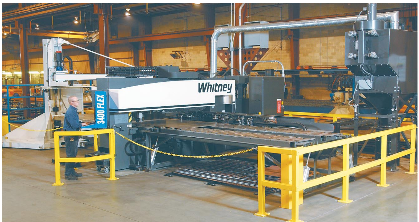
The fully integrated load/unload material handling system frees the operator for other tasks once the production cycle is initiated. The drop table on the machine's outfeed side removes completed skeletons.
