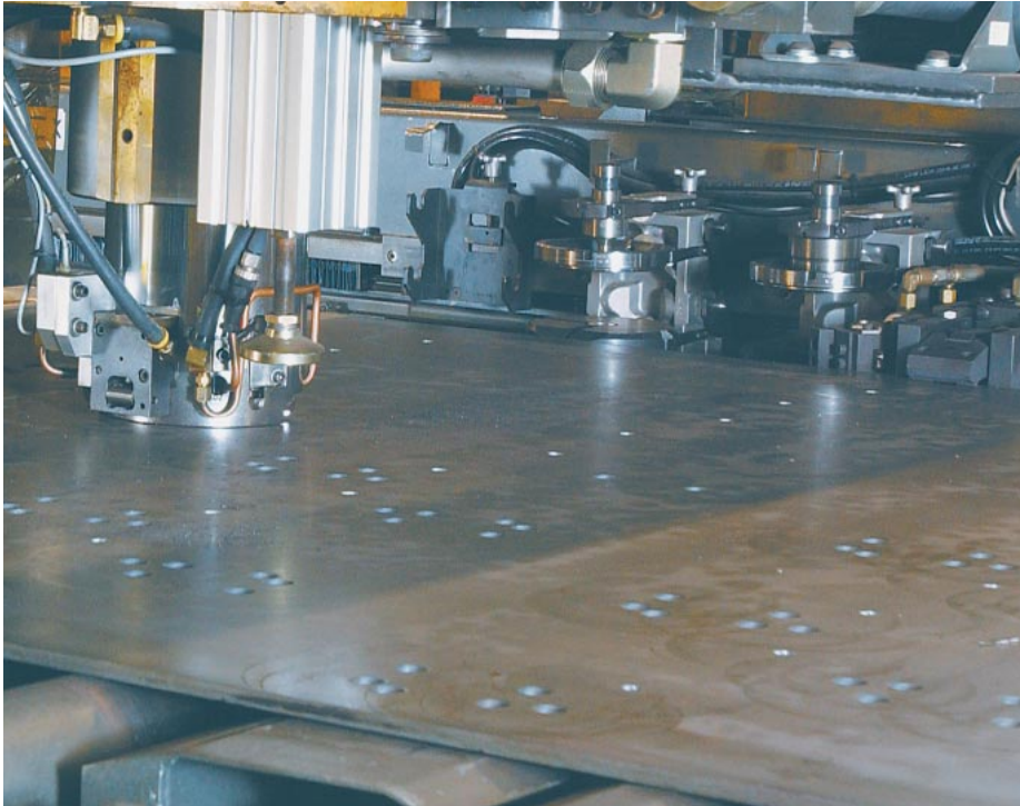
Nine tools can be positioned on the 3400 XP backrail for punching, forming or marking material up to 1" thick.
