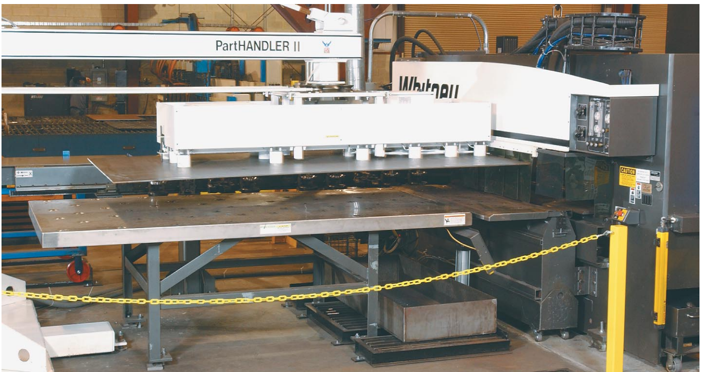
The PartHANDLER-II loads material into work clamps on the infeed side of the 3400. Plate up to 1,000 lbs. can be automatically loaded.
